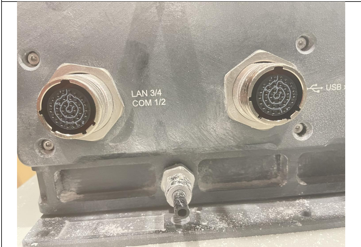
Inside view of enclosure after IP6X dust test (EUT IO)
